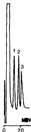
Fig. 10. Separation of transition metals in sea water. Stationary phase, IDA-silica; mobile phase, 10 mmol/l tartaric acid (pH 2.54); flow-rate, 1.0 ml/min; detection, conductivity; integration, attenuation 8. Sample: sea water spiked with (1) 5 ppm \text{Co}^{2+} , (2) 5 ppm \text{Zn}^{2+} and (3) 10 ppm \text{Cd}^{2+} .
